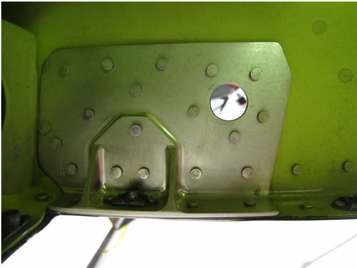
Figure 3 View Showing the Repair Fitting Installed (RH Side)
