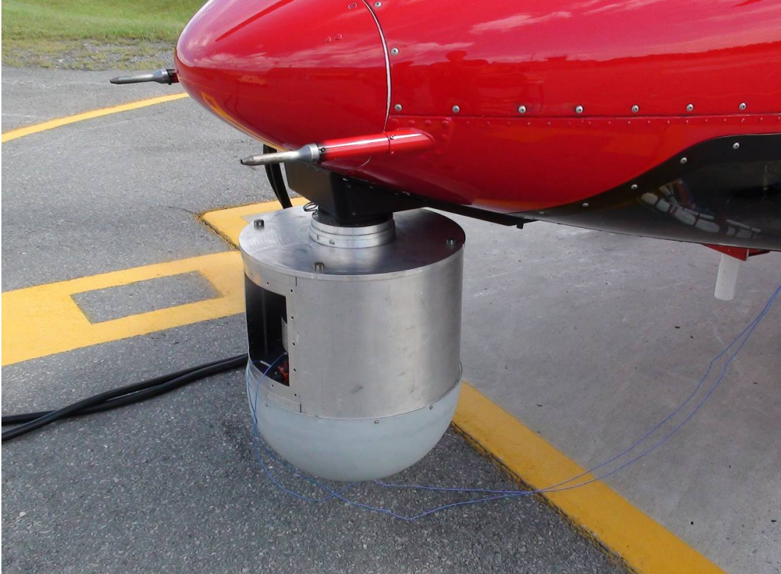
Figure 1. Typical Payload Installed onto the AFM-NM429 Nose Mount
