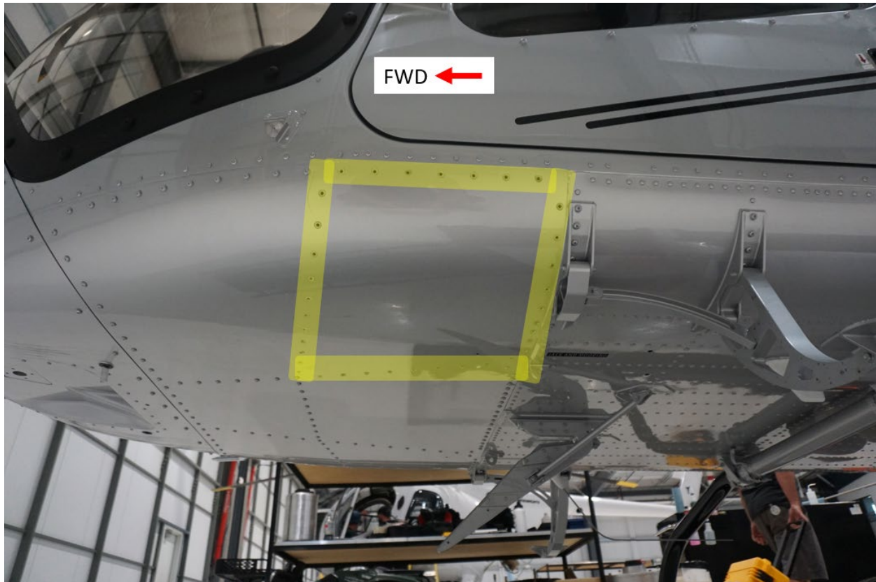
Figure 6 - View Looking at Left-Hand Nose Section of the Bell 505 Fuselage, removed fasteners shown highlighted.
