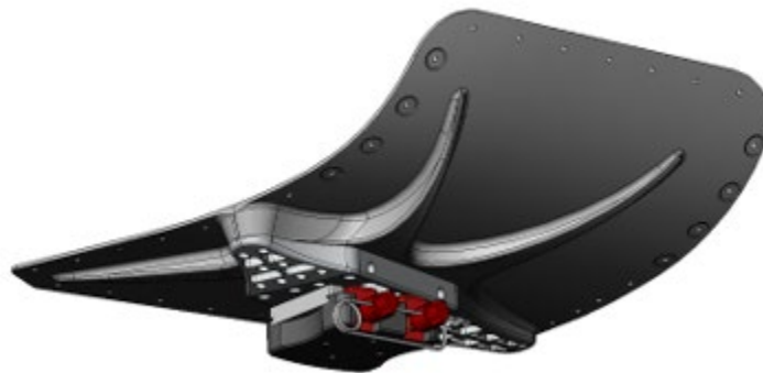
Figure 2 – AFM-505-3 Utility Downpost Mount Assembly.
