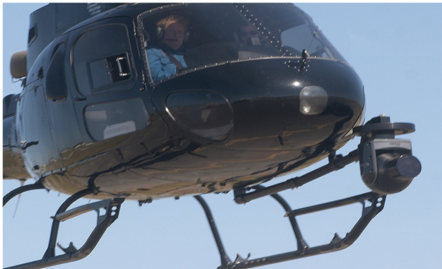
Figure 1. Single Pole with Cineflex HD (typical) – Front View
