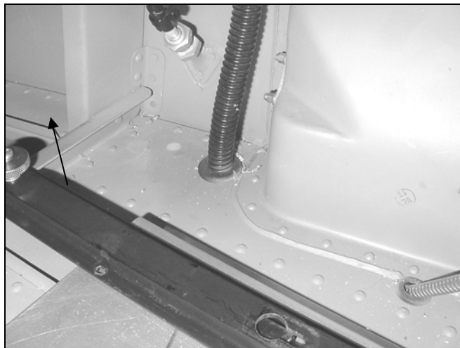
VIEW 1: TOP OF AVIONICS TRAY LOOKING AFT / OUTBOARD LEFT HAND SIDE. REMOVE RIVET AS SHOWN
