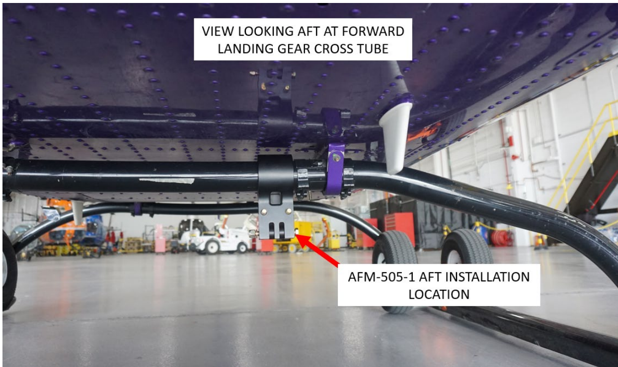
Figure 7. AFM-505-1 Aft Installation location on the Bell 505 Forward Landing Gear Cross Tube.
