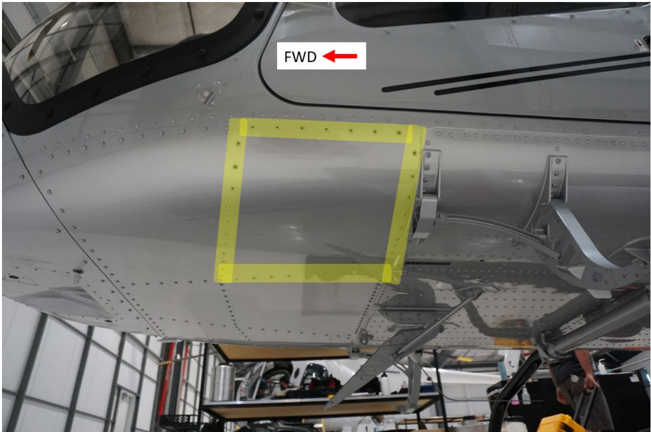
Figure 10. View Looking at Left-Hand Nose Section of the Bell 505 Fuselage, removed fasteners shown highlighted.
