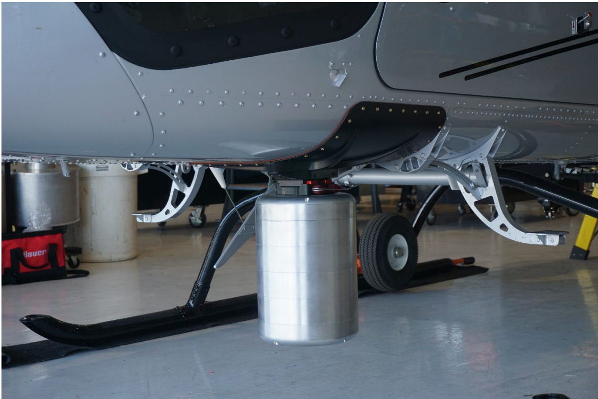
Figure 9. Installed AFM-505-3 Down Post Utility Mount, with Dummy Sensor for Reference.
