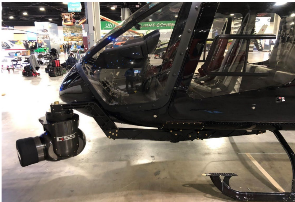
Figure 1. AFM-505-1 Beam Installation on a Bell 505 Helicopter with Sample Payload Attached
