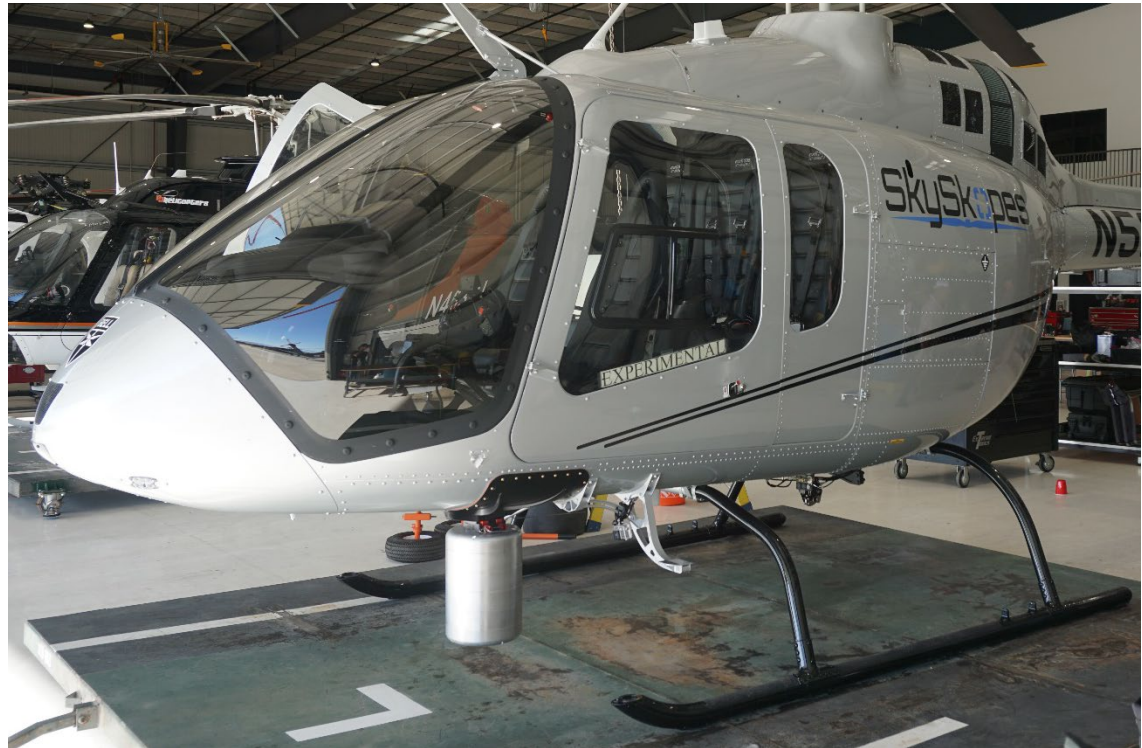
Figure 2. AFM-505-3 Downpost Installation on a Bell 505 Helicopter with Sample Payload Attached
