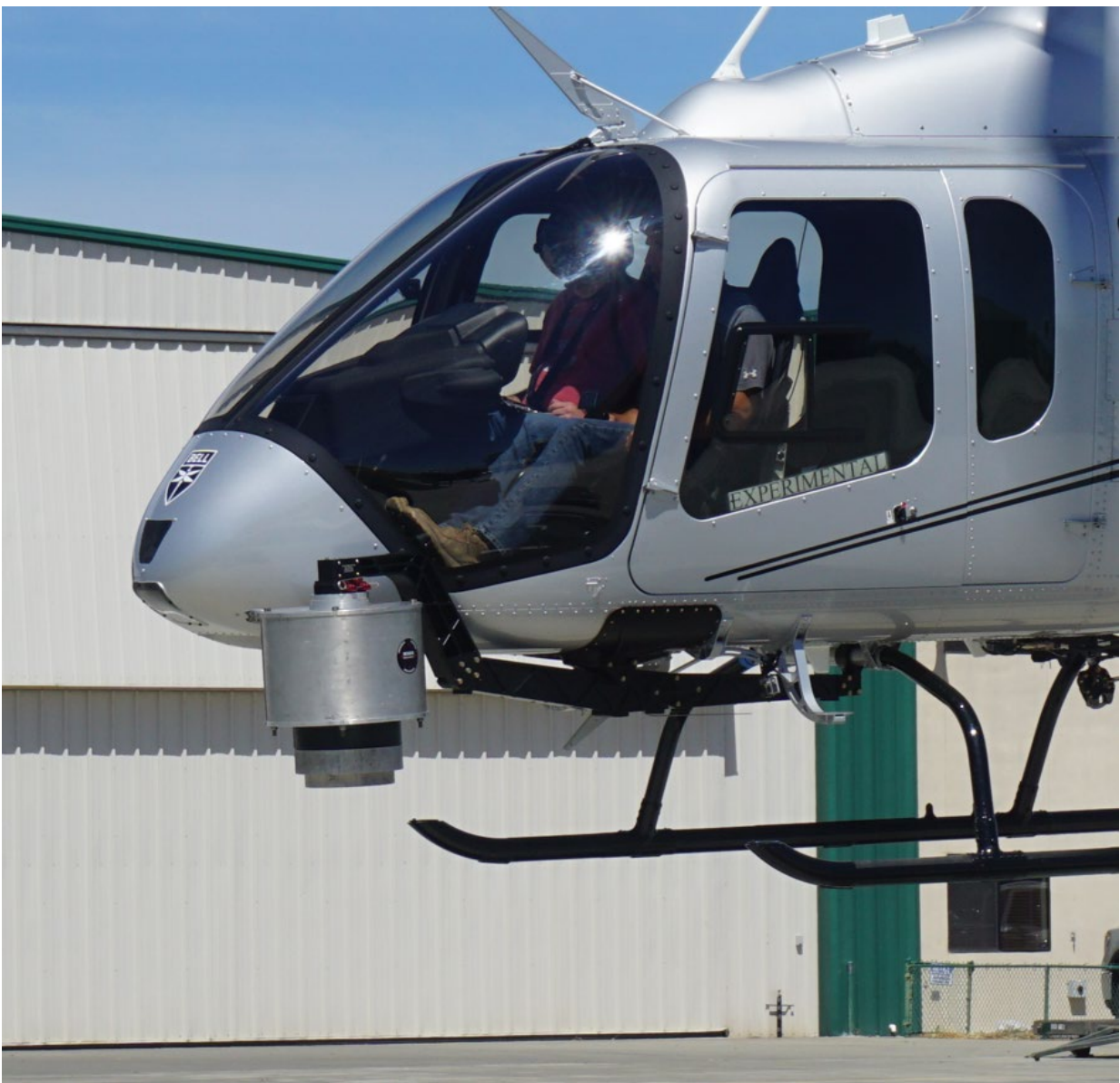
Figure 9. Installed View of the AFM-505-1 LH Nose Utility Mount
