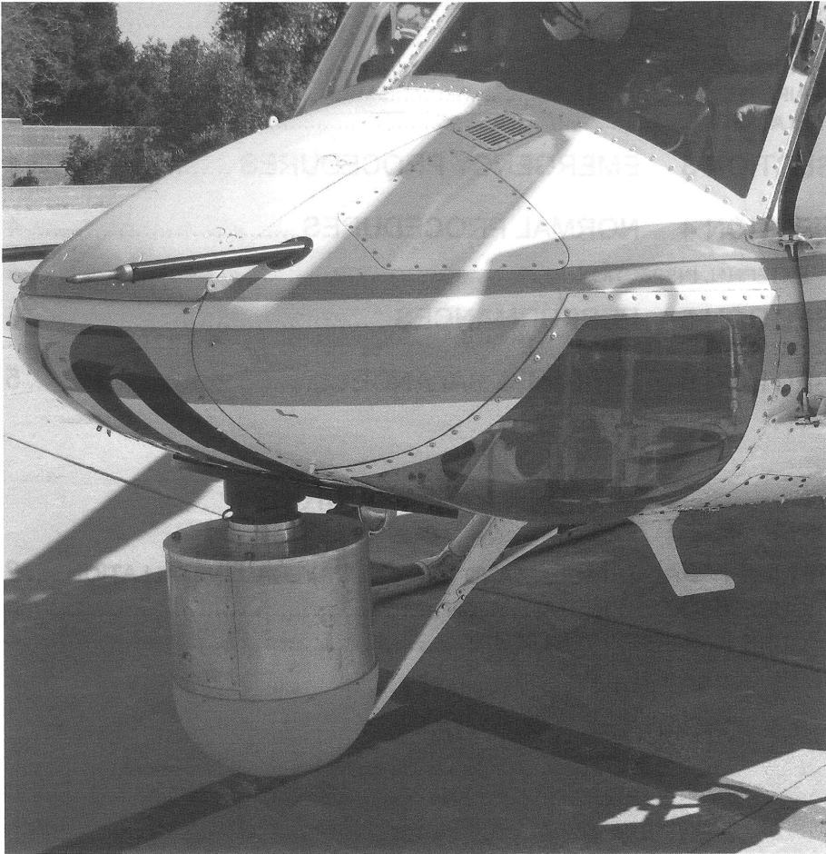
Figure 1. Front Mount and Typical Payload Installation
