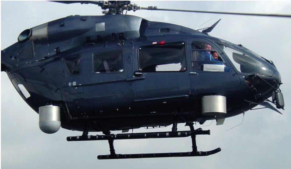
Figure 1 Camera and Light – Right Side (Typical)
