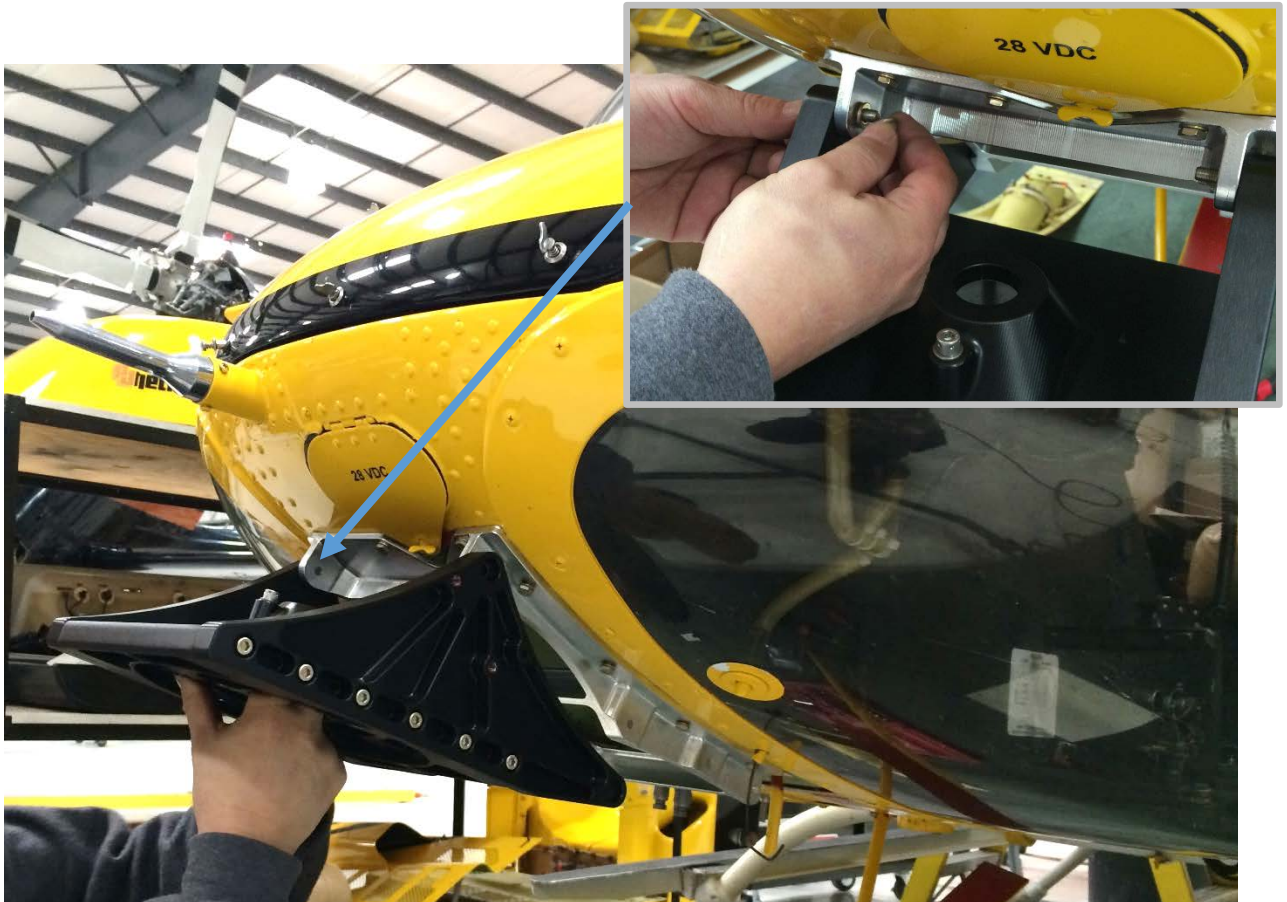
Figure 7 Installation of G1-V2 Assembly to Mounting Plate
