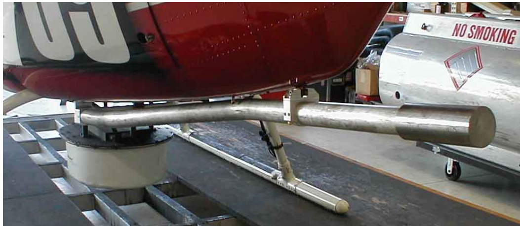
Figure 3 View Showing Option G2-1 Counterweight Assembly
