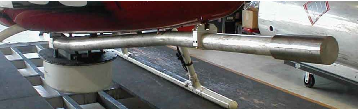
Figure 9 View Showing a Typical Installation of the G2-1 Counterweight Assy.
