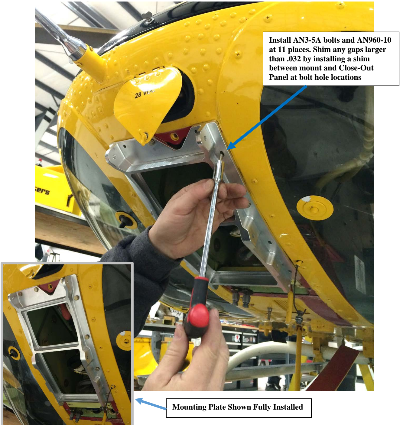
Figure 6 Installation of Base Plate (-107/-109) (Closeout Panel not shown)
