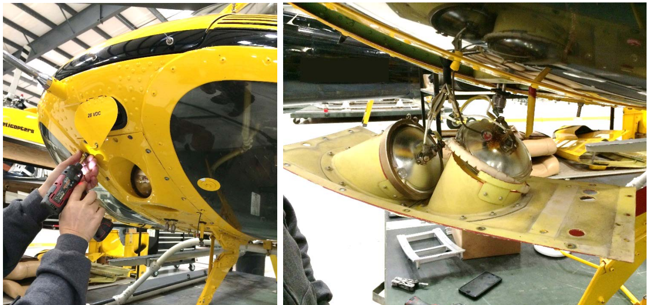
Figure 4 View Showing Removal of Landing Light (Bell 407 Shown- Bell 206 Similar)
