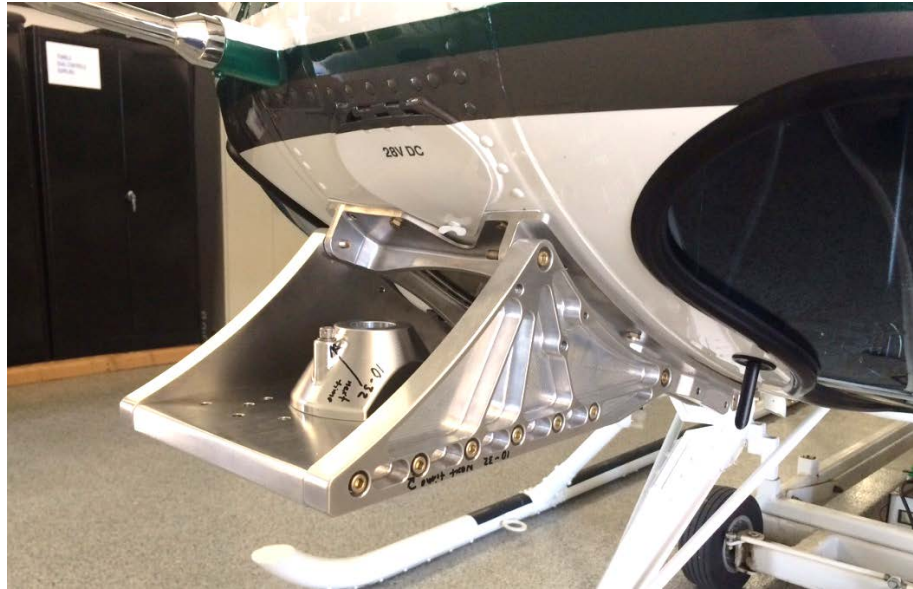
Figure 1 View Showing G1-V2-1 Installation on Bell 206
