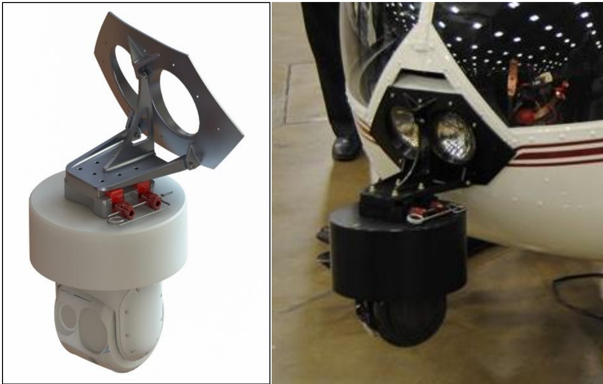
Figure 1 – (LH) Rendering of R44 Nose Utility Mount (camera shown for reference only), (RH) Picture of Mount installed on R44
