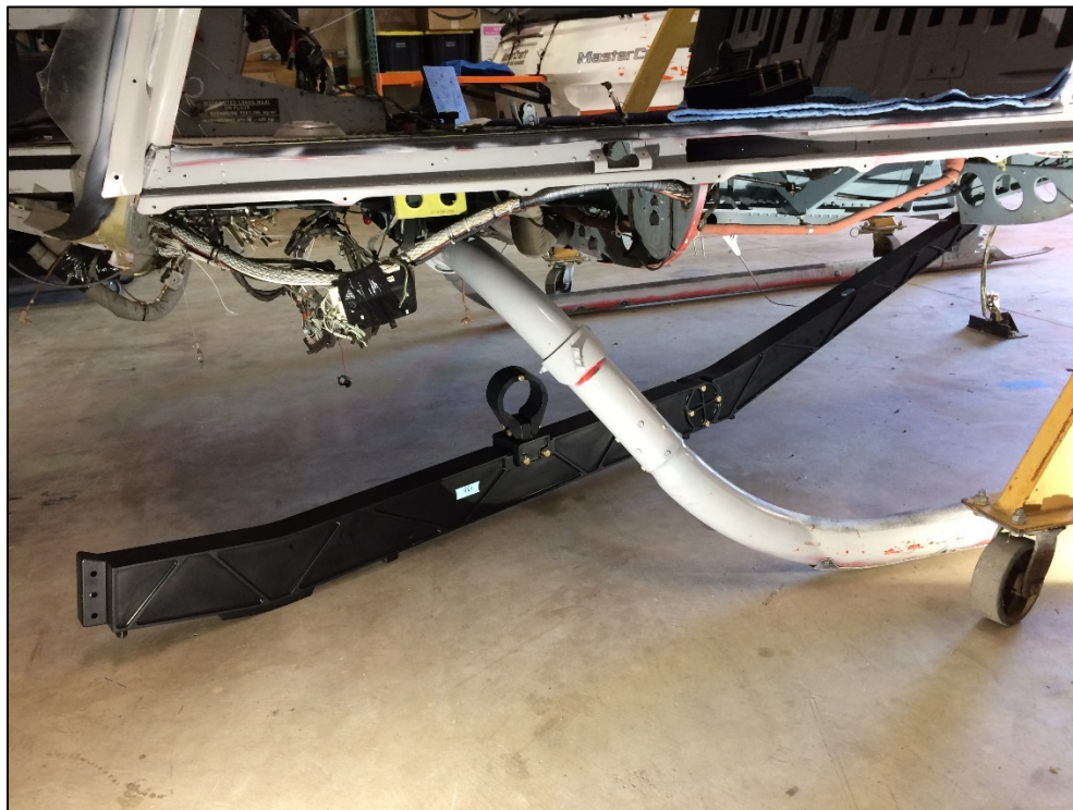
Figure 9. Forward portion of utility mount resting on the ground after aft mounting
