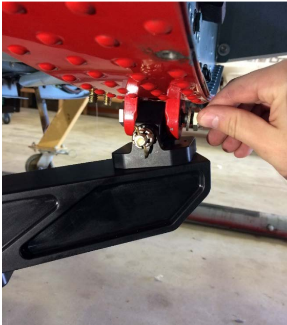
Figure 7. Aft Attachment point of utility mount attached to cargo hook hardpoint (EC130 Model B4 Shown)
