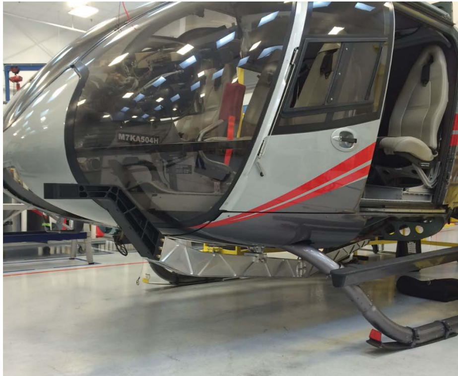
Figure 1. View Showing AFM-130 Installation on a EC130 Helicopter
