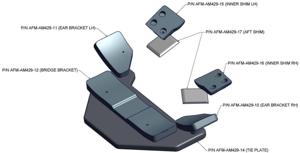
**Figure 12 - AFM-AM429-1 Drawing**
