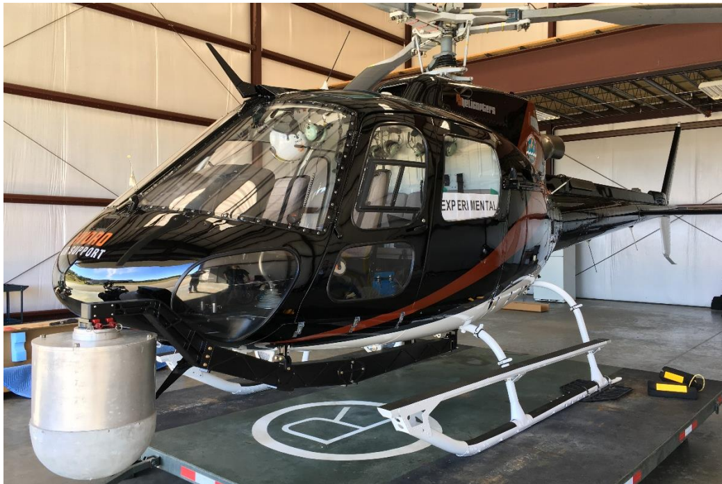
Figure 1. View Showing AFSP-V2 Installation on AS350 Helicopter
