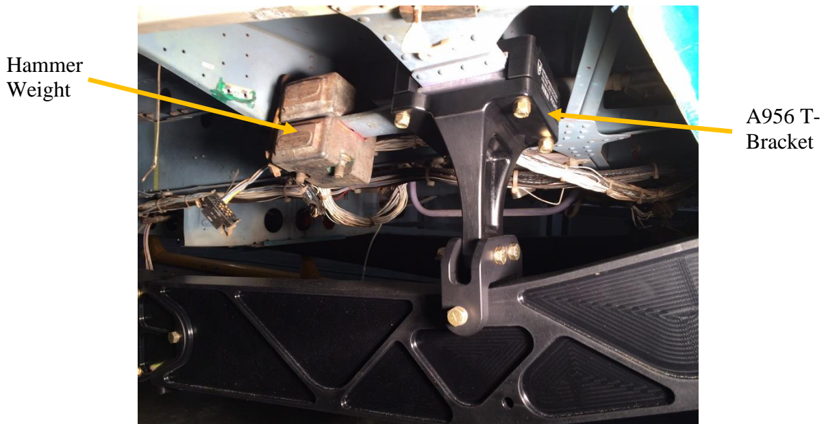
Figure 4 Installation of the Clamping A956 T-Bracket (RH Shown)
