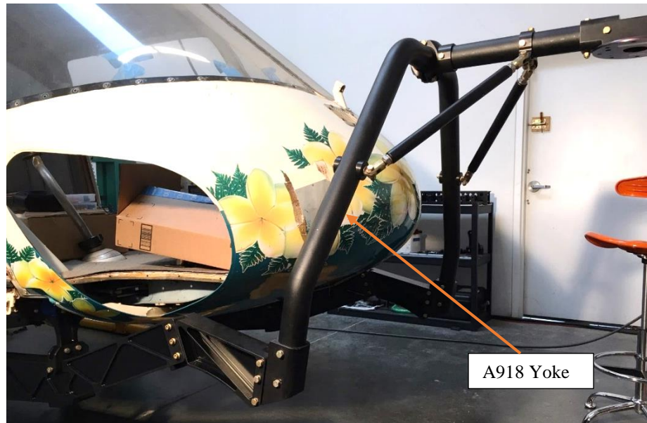
Figure 9 Installation of the A918 Yoke for the Dual Pole Configuration
