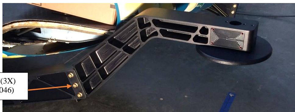
Figure 7 Installation of the Forward Arm for Single Pole Configuration
