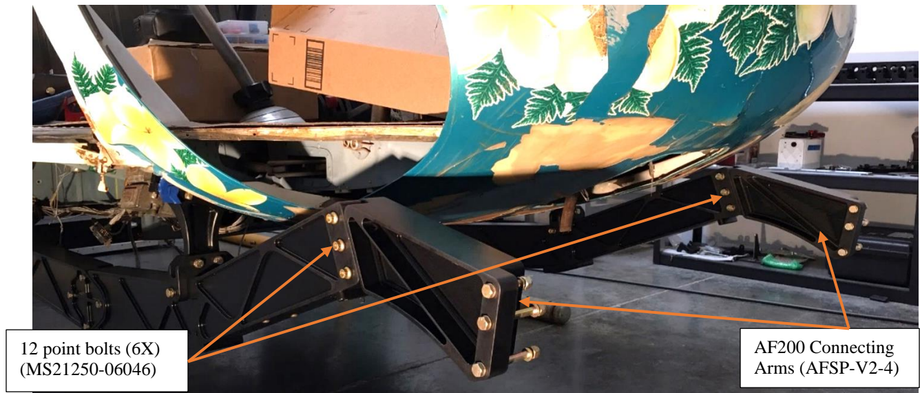
Figure 8 Installation of the AF200 Connecting Arms for the Dual Pole Configuration
