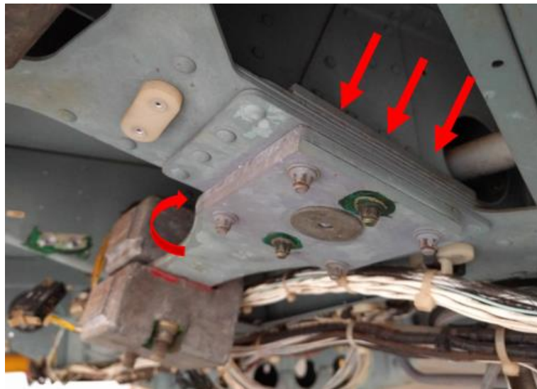
Figure 2. Location of A953-1 and A956 Assembly installation on aircraft hammer weight fitting
