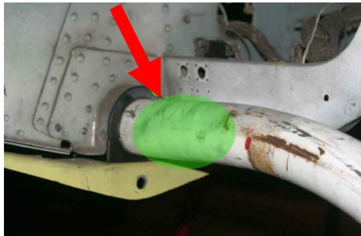
Figure 3. Location of rear clamp installation on forward cross tube
