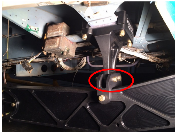
Figure 1. Forward Attachment point and T-Bracket of the AFSP-V2
