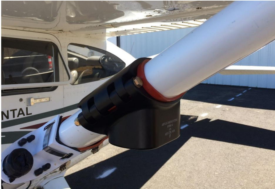
Figure 1. View Showing the AFWM-1 Installation on a Cessna 182
