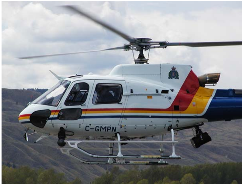
Amtech Mount – AMT 342 Kit - Installed on an AS350 Helicopter
