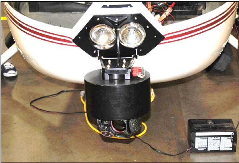
Figure 1. R44 Nose Utility Mount installation
